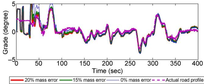
Fig. 6. Demonstration of the sensitivity of the grade estimator to errors in mass estimate.
