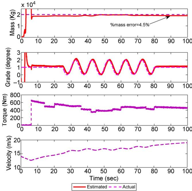
Fig. 3. Estimation results for simulated data when the grade is sinusoidally varied.
