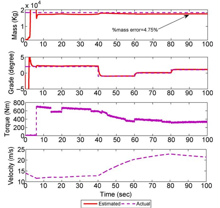
Fig. 2. Estimation results for simulated data when the grade is varied in steps.
