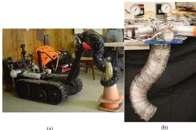
Fig. 1. In (a), the OctArm continuum manipulator grasps a traffic cone. Shown here, it replaces the end-effector of a Foster-Miller Talon robot. In (b), the two-section Air-Octor continuum robot is shown.
