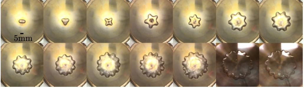
FIG. 2. Experimentally observed star oscillations in water drops with mode numbers  $n = 2$ –15 on  $R_s = 83.3$  mm plate.
