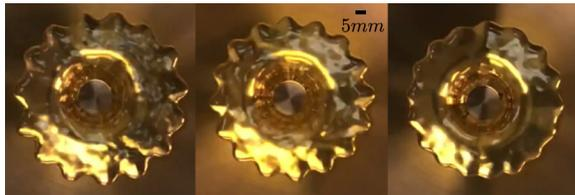
FIG. 6. Drop oscillations exhibit mode numbers  $n = 15$ – $17$  on the toroidal geometry using water.
