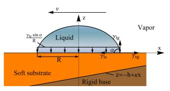
FIG. 2. Definition sketch showing a two-dimensional liquid droplet of radius *R* in contact with the free surface of a solid substrate with a variable thickness  $-h + \kappa x$ . The drop applies surface tension forces on the solid at the contact line x = R and bulk fluid pressure along the length of the droplet
