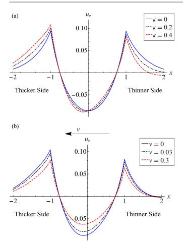
FIG. 3. Vertical deformation  $u_z$  of a soft substrate at the liquidsolid interface z = 0 as it depends upon (a) thickness gradient  $\kappa$ ( $\Lambda = 1$ ,  $\Gamma_s = 1$ ,  $\Gamma_l = 2$ , v = 0) and (b) dimensionless velocity v( $\Lambda = 1$ ,  $\Gamma_s = 1$ ,  $\Gamma_l = 2$ ,  $\kappa = 0.3$ , n = 0.5).
