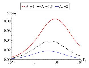
FIG. 5. Driving force  $\Delta \cos \alpha$  plotted against the elastocapillary number  $\Gamma_l$  with different aspect ratios  $\Lambda$ . Here,  $\nu = 0.5$ ,  $\Gamma_s = 0.5\Gamma_l$ ,  $\kappa = 0.3$ ,  $\nu = 0$ .
