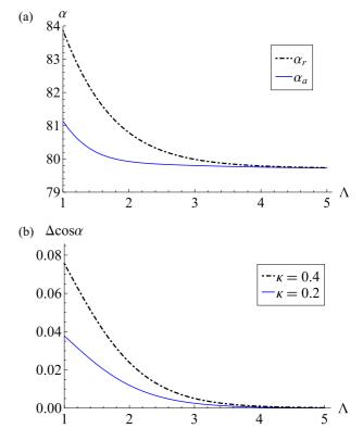
FIG. 4. (a) Advancing  $(\alpha_a)$  and receding  $(\alpha_r)$  receding contact angles of the drop in degrees plotted against the aspect ratio  $\Lambda$ . Here  $\kappa = 0.25$ . (b) Dimensionless driving force  $\Delta \cos \alpha$  against  $\Lambda$  for different thickness gradient  $\kappa$ . In both figures, v = 0,  $\Gamma_s = 0.5$ ,  $\Gamma_l = 2$ .
