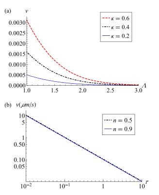
FIG. 7. (a) Dimensionless velocity v plotted against aspect ratio  $\Lambda$  with different thickness gradient  $\kappa$ . Here,  $\Gamma_s = 1$ ,  $\Gamma_l = 2$ , n = 0.6. (b) Velocity in  $\mu$ m/s plotted against relaxation timescale  $\tau$  with different power-law exponent n. Here,  $\Lambda = 1$ ,  $\Gamma_s = 3$ ,  $\Gamma_l = 6$ ,  $\kappa = 0.4$ ,  $R = 10 \mu$ m.
