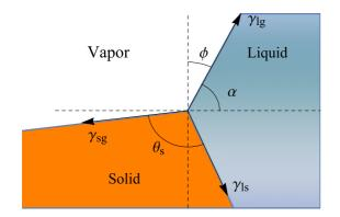
FIG. 1. Orientation of the triangular cusp formed at the tip of the wetting ridge. Macroscopic solid-liquid contact angle  $\alpha$  changes as the cusp rotates through a tilt angle  $\phi$  which depends upon the elastic response of the solid substrate. The solid angle formed inside the cusp is denoted as  $\theta_s$ .
