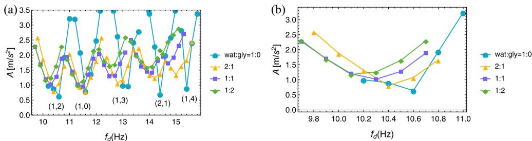
FIG. 6. Acceleration  $A$  against driving frequency  $f_d$  for glycerol/water mixtures with height  $H = 22$  mm and pinned contact-line illustrating (a) the full frequency scan and (b) only the (1,2) mode.
