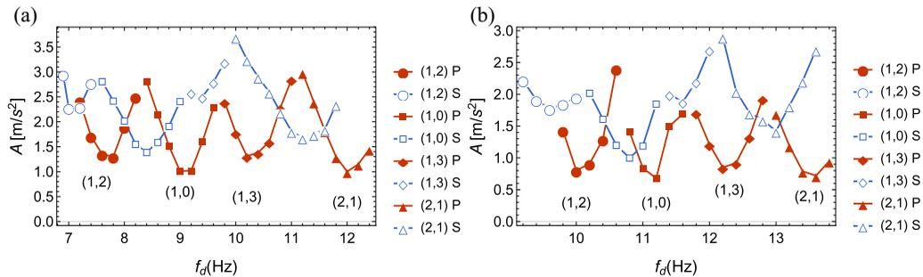
FIG. 5. Acceleration  $A$  against driving frequency  $f_d$  for the Triton/water mixture contrasting the free-sliding (S) and pinned (P) contact-line condition for fluid height (a)  $H = 7$  mm and (b)  $H = 22$  mm.
