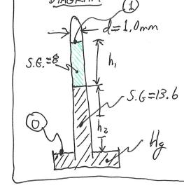
$101,325 \text{ Pa} = 0 \text{ Pa} + (8)(1000 \frac{kg}{m^3})(9.81 \frac{m}{s^2})(0.637m) + (13.6)(1000 \frac{kg}{m^3})(9.81 \frac{m}{s^2})$  $50/ving \rightarrow h_z = 0.385 m = 38.5 cm$   $h_z = 38.5 cm$
