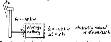
ASSUMPTIONS: (1) The battery is a closed system. (2) The work and heat transfer rates are constant.
