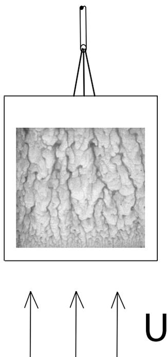
FIG. 3. Top view of the experimental facility showing the surfactant rake and the water tank. A sample IR image is superimposed on the surface of the water showing the region that was imaged.
