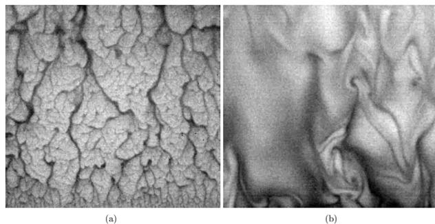
FIG. 4. IR images of a water surface at a wind speed  $U=2$  m/s. (a) The water surface is free of surfactants. (b) The water surface is completely covered with a surfactant monolayer. In both images the heat flux leaving the tank is approximately  $625$  W/m<sup>2</sup>. The flow of air is from the bottom of the image to the top.
