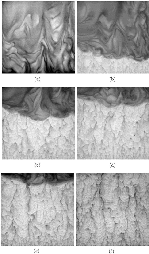
FIG. 5. IR imagery of the water surface during the cleaning process for a wind speed  $U=3$  m/s. (a) Before cleaning. Time after initiation of cleaning: (b)  $t=56$  s, (c)  $t=117$  s, (d)  $t=147$  s, (e)  $t=165$  s, and (f)  $t=325$  s.
