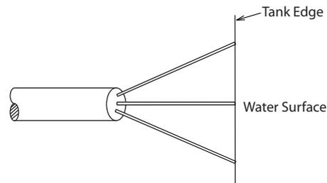
FIG. 1. The surfactant tube rake viewed from above, showing the three microbore tubes, connected to a larger diameter tube.
