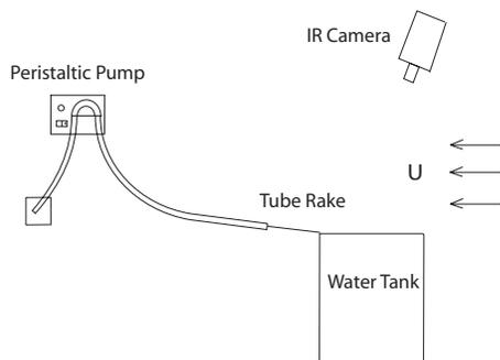
FIG. 2. Experimental facility used to test the surfactant tube rake shown in Fig. 1. The rake is located at the downstream end of the glass tank and at the air/water interface.
