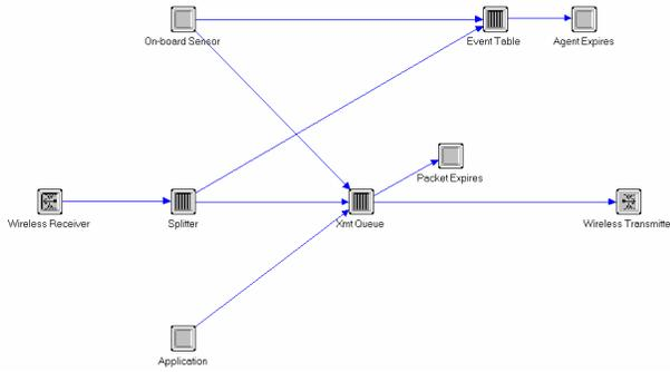
Figure 1: Wireless sensor node model in OPNET
