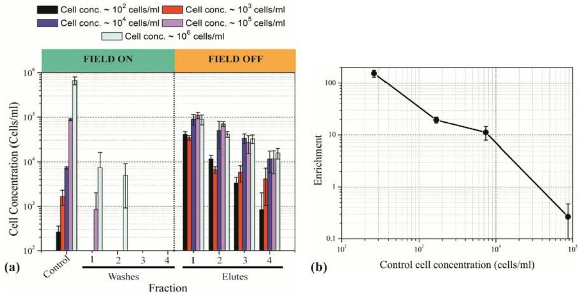
Figure 2: (a) Results of carbon electrode DEP of the yeast cells with different cell concentration at 20 V<sub>pp</sub>, 100 kHz and 10  $\mu$ l/min; (b) Enrichment for different cell concentration
