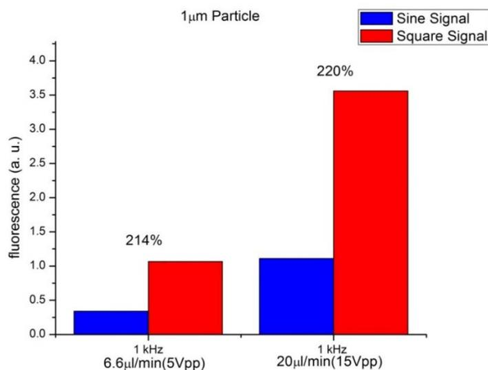
Figure 6. Results for the same relation Voltage-Flow Rate
