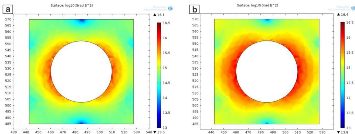
Figure 3. a) Modeling of  $gradE^2$  for 5 V<sub>RMS</sub> sinusoidal signal. b) Modeling of  $gradE^2$  for 5 V<sub>RMS</sub> square signal.
