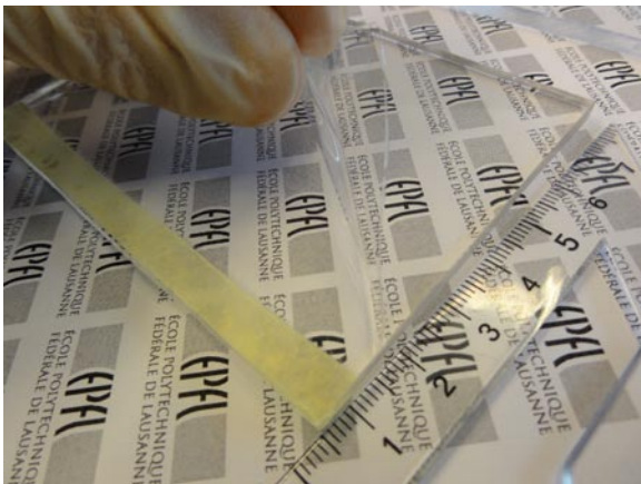
Figure 5. Release of the PDMS film from one of the plates after it has been cross-linked by heating
