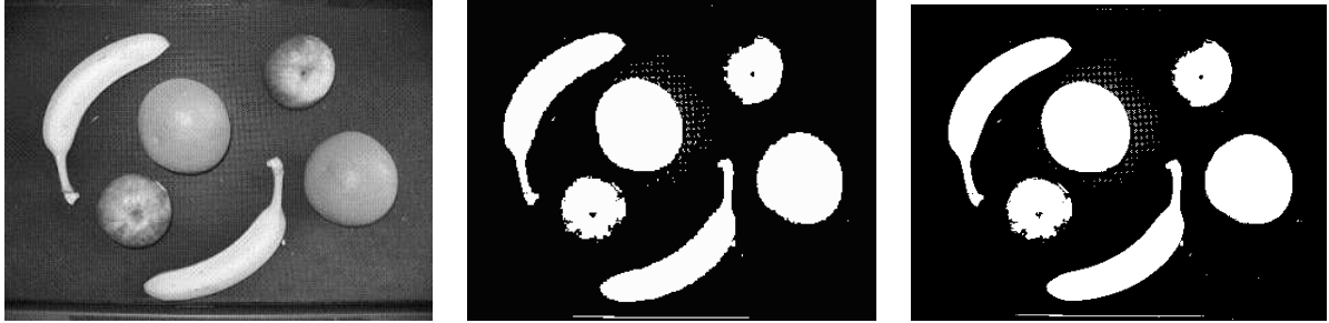
Figure 2.5: From left to right: Input image, output of Rider-Calvard, and output of Otsu. The outputs are almost indistinguishable.
