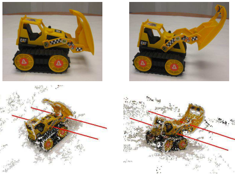
Fig. 12. Occlusion-aware reconstruction of an articulated object with multiple axes. For the two configurations, 111 and 134 images, respectively, were captured.
