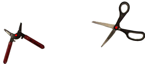
Fig. 6. Revolute axis estimation of pliers (left) and scissors (right) in 2D found by our method. The red dot indicates the estimated axis of rotation.
