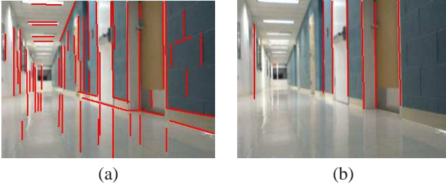
Figure 4. (a) Line segments detected by Canny edge detector followed by line detection. (b) Candidate door segments retained after applying multiple tests to the segments.
