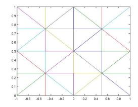
Figure 5.1: Computational mesh corresponding to h = 1/4.
