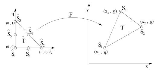
Figure 2.1: Mapping of the reference triangle  $\hat{T}$  to the triangle T.
