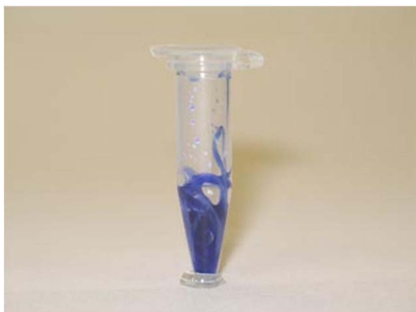
Fig. 4. Nylon fibers with attached BVBlue reagent change color from white to blue in the presence of 0.06 U of sialidase from Arthrobacter ureafaciens after treatment with 0.1 M sodium hydroxide. (For interpretation of the references to colour in this figure legend, the reader is referred to the web version of this article.)
